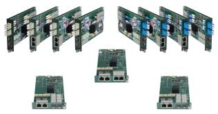
The modular network TAP is ideal for network monitoring and access with your active in-line appliances. Bypass TAPs provide complete, fail-safe protection for in-line appliances like firewalls, intrusion prevention systems (IPS), data leakage protection (dlp), web content filters, and more.
